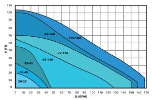
The ecocirc XL delivers high pump head performance for applications with many pressure-consuming components but low flow requirements.
