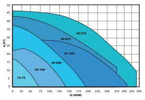
The ecocirc XL also delivers high flow rates for hydronic systems with changing flow requirements.
