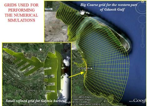
Fig. 3: NIVA model was buildt up with a coarser grid for the bay of Gdansk and finer grid for the Gdynia harbour
