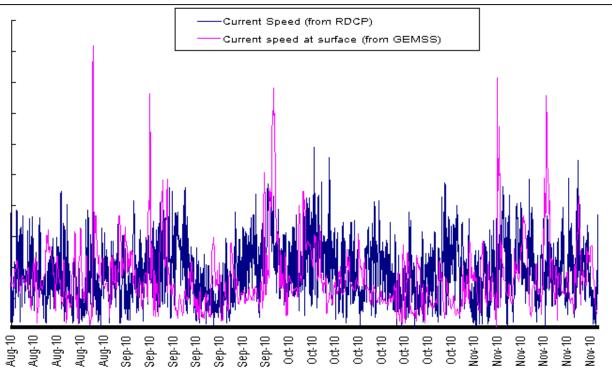
Fig. 5: Surface currents at the harbour entrance measured with RDCP-600 (blue) and from model (pink)
