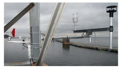
Fig. 6B: Wind and Weather sensors at harbour entrance
