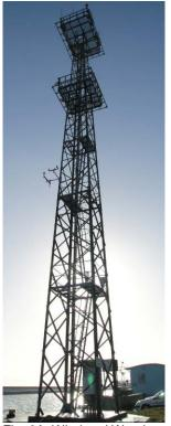
Fig. 6A: Wind and Weather sensors installed 15m above ground level
