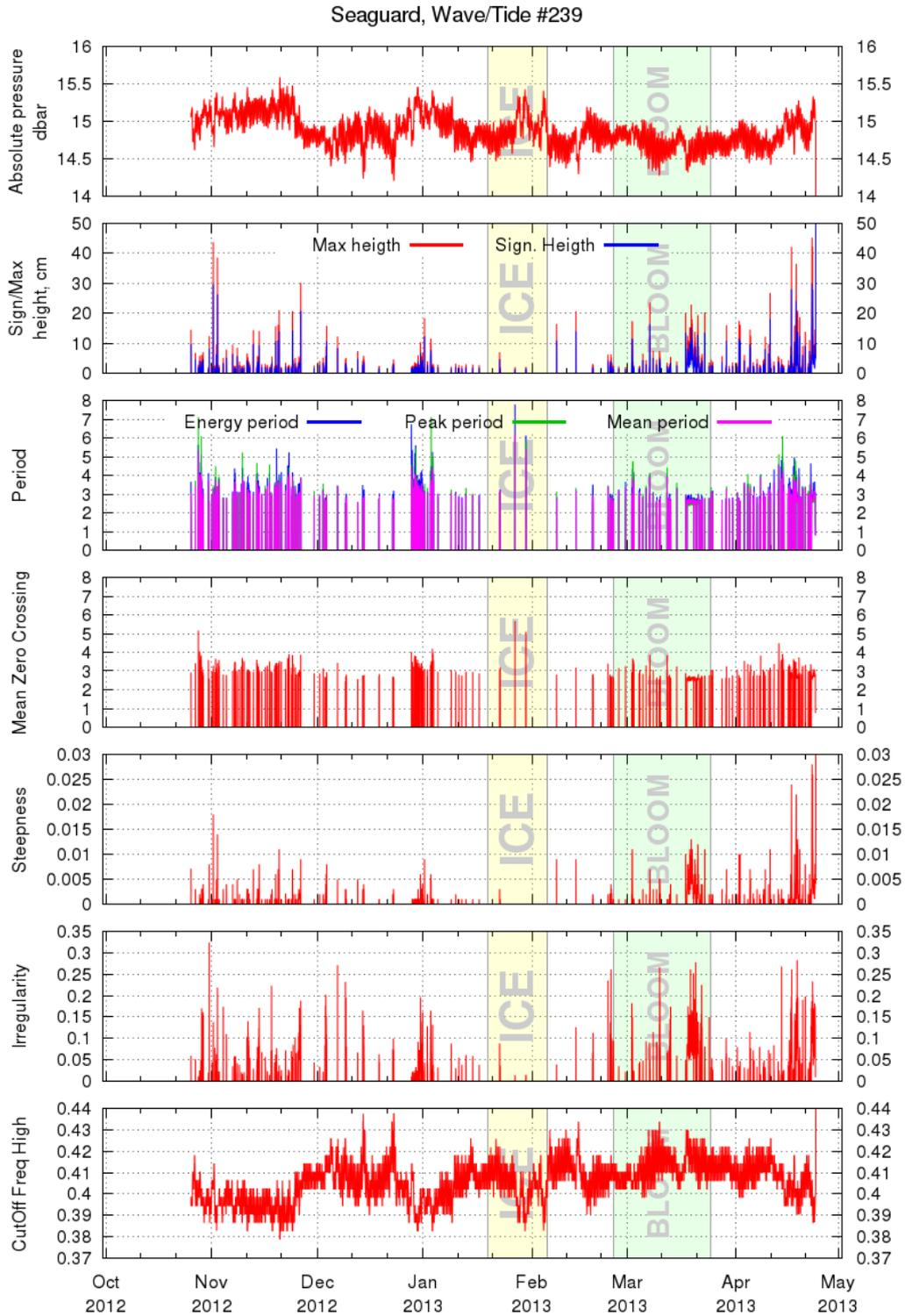
Figure 15: Seaguard Wave/Tide sensor #239 data. A period with strong waves in mid-March 2013 at the end of the bloom.
