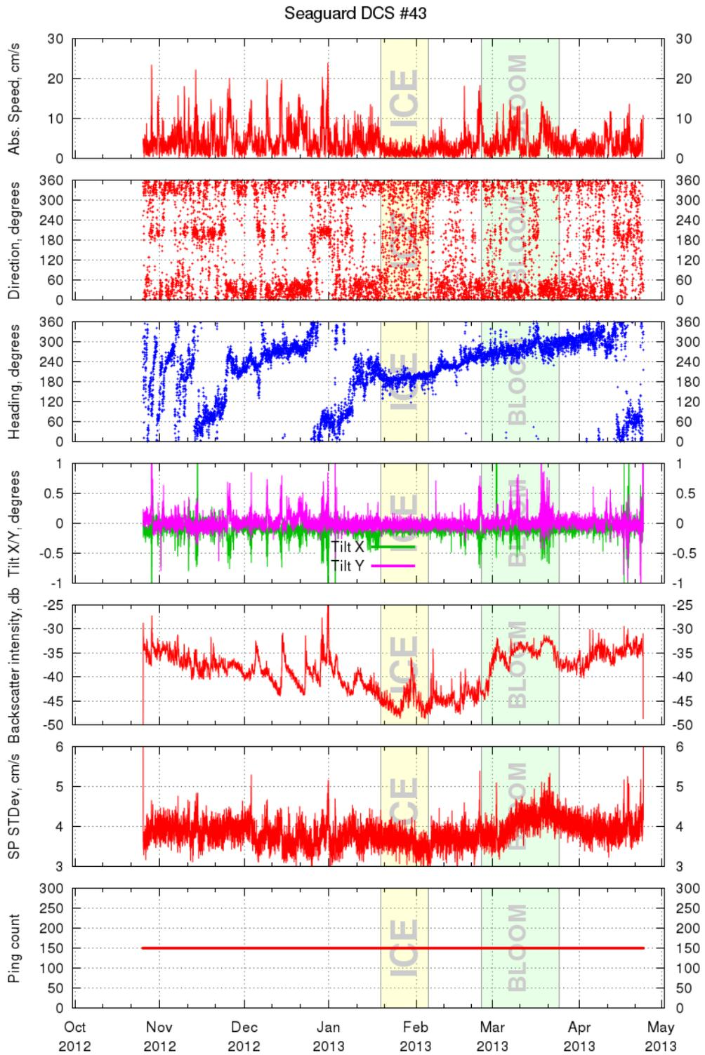
Figure 14: Seaguard DCS #43 data. Weak currents, chaotic direction and quite stable heading under ice.
