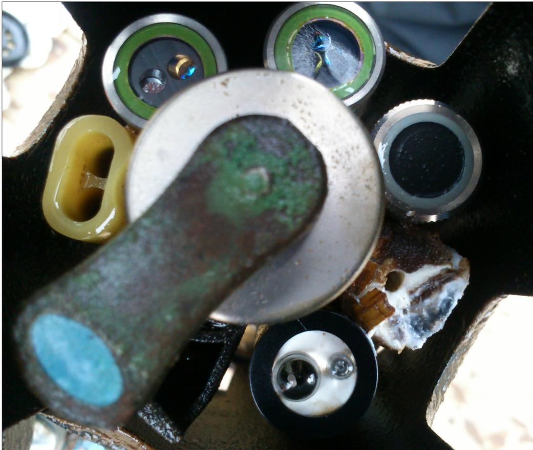
Figure 3: EXO2 sensor tips on recovery, before any washing or cleaning. Sensor sockets were populated with: C/T, fDOM, TA/BGA, ODO, sacrificial anode, and pH/ORP sensor. All sensors looked nice and clean after 6 months in sea water due to wiper brush cleaned working surfaces. Some consumption of sacrificial anode metal occurred.
