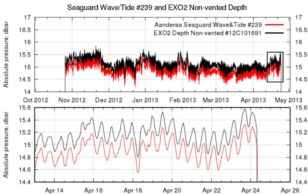
Figure 9: EXO2 Pressure. Periodical oscillations due to tidal movements of sea level (shown on lower panel). Permanent offset of approx 22 cm suggests difference between depth levels of pressure sensors on EXO2 and Aanderaa Seaguard.
