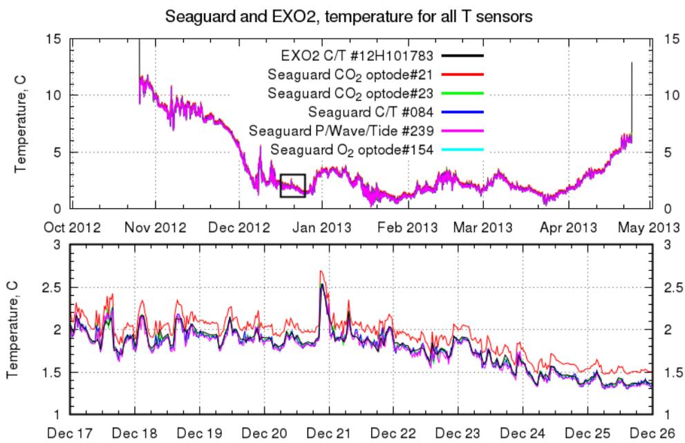
Figure 7: EXO2 and Seaguard, temperature from all sensors. pCO<sub>2</sub> optode #21 readings were always higher by 0.15 C. All other T sensor readings seem to agree very well.
