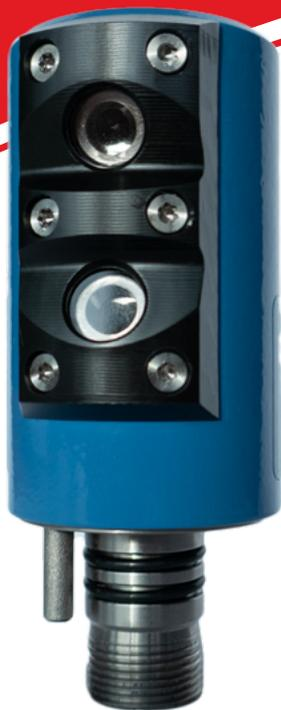
**Turbidity Sensor 4296 is a compact fully integrated sensor for measuring optical backscatter in water. It is designed to be used with SeaGuard or SmartGuard data logger using AiCaP CANbus or as stand-alone sensor using RS-232**
