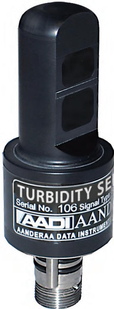
The Turbidity sensor 4640 is based on the seapoint turbidity meter. The sensor detects light scattered by particles suspended in water.
