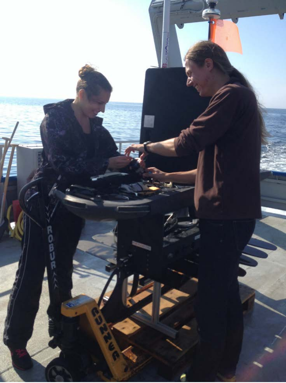
pCO 2 and O 2 optodes on IFM-Geomar wave glider during PhD course
