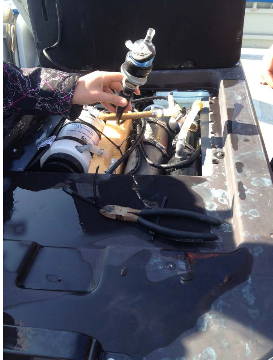
pCO 2 and O 2 optodes on IFM-Geomar wave glider during PhD course
