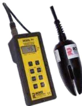
The Royce Model 711 Portable Suspended Solids/ Interface Level Analyzer is a rugged, waterproof instrument designed for the rigors of remote sampling. The meter provides reliable operation in waste treatment plants, rivers, lakes and other aqueous systems. The meter will read in either grams per liter when in the suspended solids mode or relative density percentage while in the interface level mode of operation.
