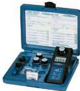
Small portable turbidity meter as per DIN ISO / US EPA for nephelometric measurements in quality control and environmental monitoring.
