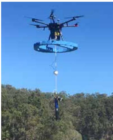
Xylem introduces its first portable autonomous water quality measurement system designed specifically for fast, safe access to challenging sites.
