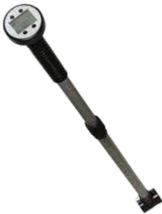
Global Water's FP111, FP211 and FP311 Flow Probes are highly accurate water velocity instruments for measuring flows in open channels and partially filled pipes. The water velocity probe consists of a protected water turbo prop positive displacement sensor coupled with an expandable probe handle ending in a digital readout display. The water flow meter incorporates true velocity averaging for the most accurate flow measurements.
