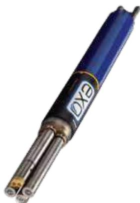
The EXO advanced water quality monitoring platform includes the versatile multiparameter EXO1 sonde for estuarine, surface water, or ground water applications.
