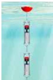
The RCM Blue is a rugged self-recording current meter with Bluetooth for communications and data retrieval. The instrument uses a true vector-averaging sensor for measuring current speed and direction in salt or fresh water, and a battery container with battery capacity up to 70Ah.
