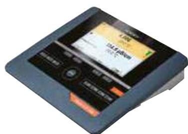
The YSI MultiLab line includes the 4010-1 (single channel), 4010-2 (dual channel) and 4010-3 (three channel) instruments that provide easy-to-use and -calibrate menu-driven operation ideal for the laboratory.
