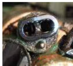
CT sensor prior to antifouling measures. Cleaning brush couldn't reach inside sensor.
