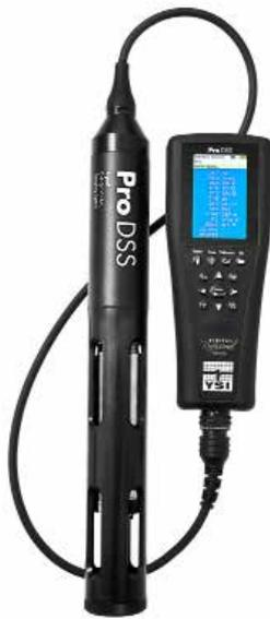
The YSI ProDSS (digital sampling system) is a portable water quality multiparameter instrument for the measurement of several critical parameters - dissolved oxygen (optical), total algae, turbidity, pH, ORP, conductivity, specific conductance, salinity, TDS, resistivity, TSS, ammonium, ammonia, chloride, nitrate, depth (optional), temperature and GPS coordinates.
