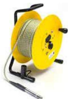
The Water Level Sounder meets or exceeds federal specification US GGG-T-106E (USA) or EEC CLASS II (Europe) for a guaranteed accuracy of 0.008%. It uses a full depth-rated stainless steel and teflon probe that is 16 mm in diameter with sensor electronics encapsulated in a water and dust proof housing.
